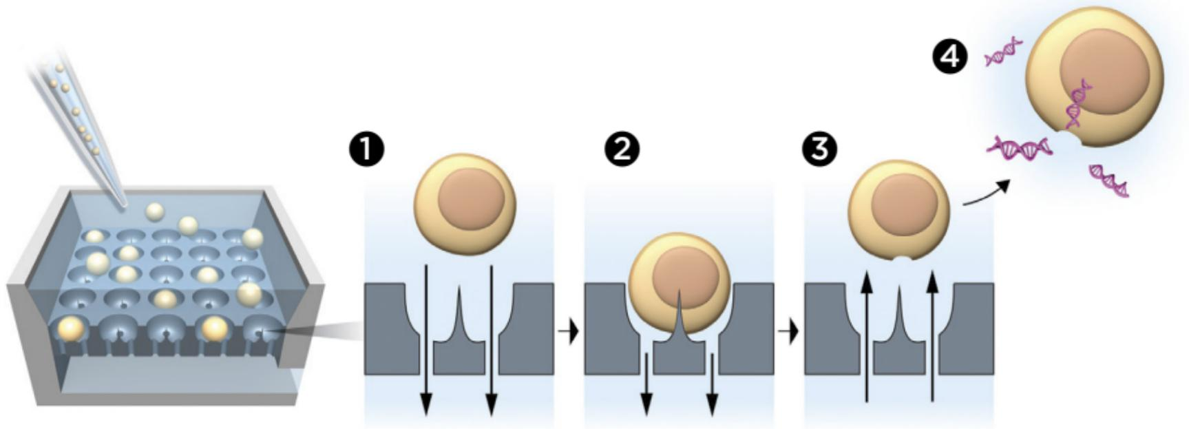
**SPIKED CELLS:** Cells in suspension are pipetted into a reservoir with an array of cell-size wells each containing a single spike. Microfluidic channels running through the wells generate a suction force that draws cells into individual wells **1**, where the spikes pierce the cell membranes **2**. The flow is reversed to release the cells **3**, which are then mixed with the DNA of interest **4**. The DNA diffuses into the cells via the temporary pores, which then close up on their own.
