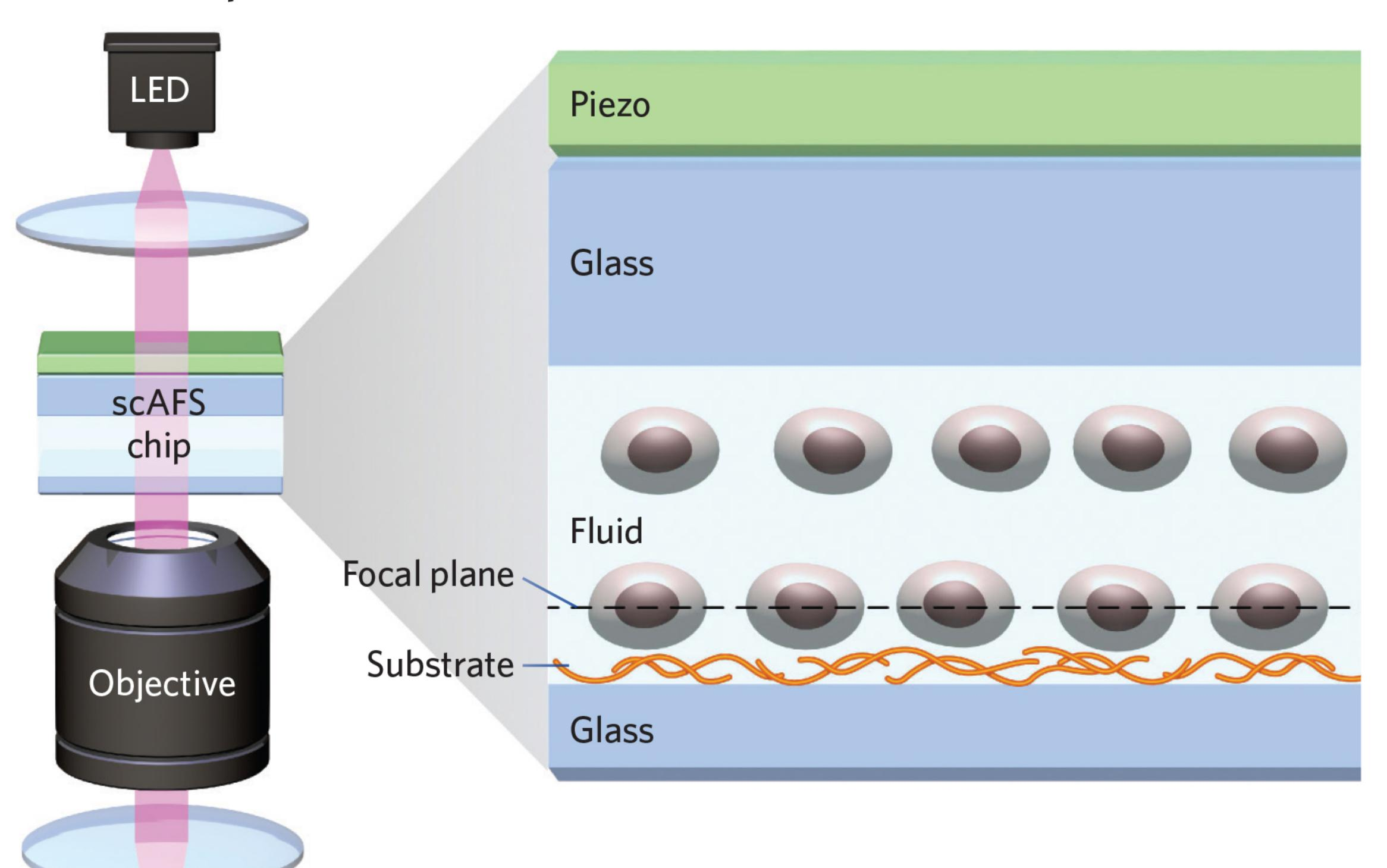
**GET UP, GET ON UP**: A piezo-produced acoustic standing wave fills the single cell acoustic force spectroscopy (scAFS) chamber, forcing non-bound cells to move up to the wave's nodal plane and out of the microscope's focal plane.
